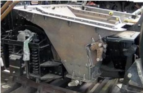
**What is an ashpan?** The ashpan is a steel receptacle mounted underneath the firebox and below the grates. It catches and collects hot embers, ashes and other solid combustion waste as it falls through the grates. It is usually fitted with dampers to adjust the airflow through the fire.
